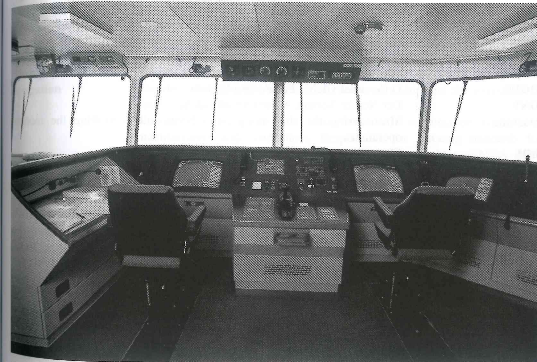
Figure 6.14 A typical integrated bridge VMS-VT installation. (Reproduced courtesy of Litton Marine Systems.)
