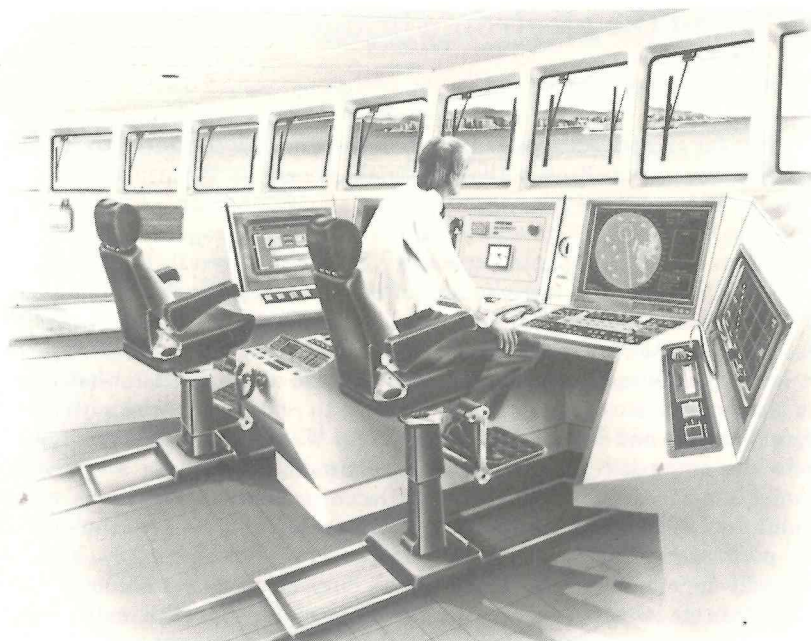
Fig. 18. Artist's impression of the integrated bridge, including 2690 BT ARPA, CVP 3500 and MNS 2000 with LSR 4000 screen (courtesy Racal Marine Electronics Ltd)
