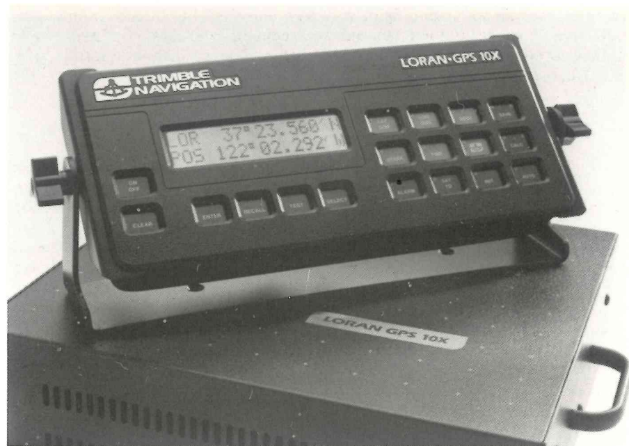
Fig. 24. An integrated GPS/Loran C receiver (courtesy of Trimble Navigation Ltd)
