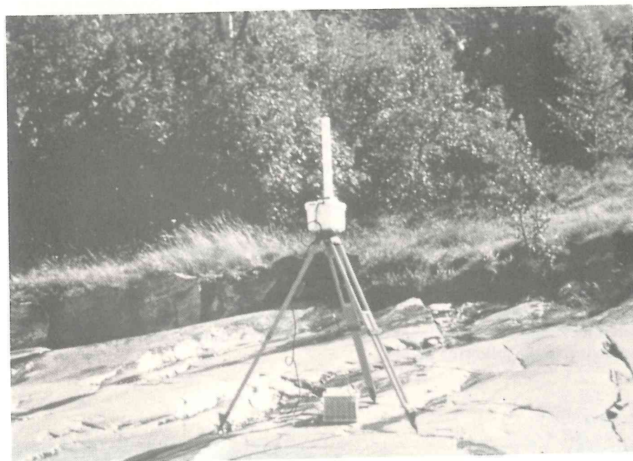
Fig. 53. Micro-fix beacon (courtesy of Racal Marine Systems Ltd)
