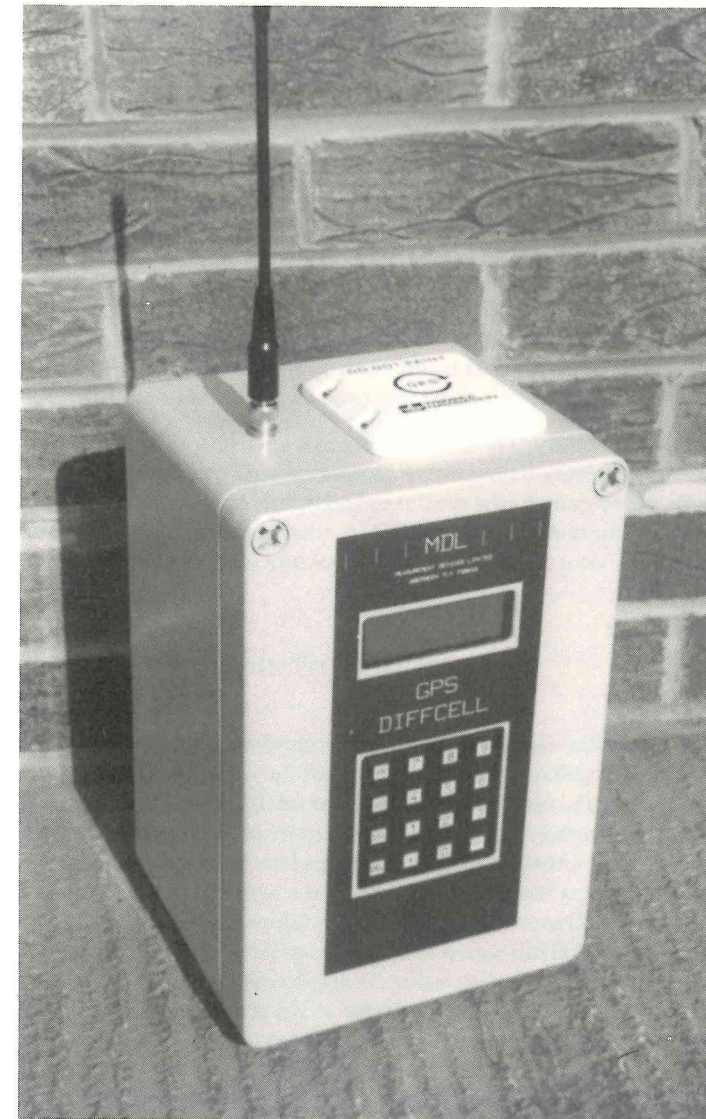
Fig. 37/38. Diffcell—a combined GPS receiver and VHF transmitter (courtesy Measurement Devices Ltd)
