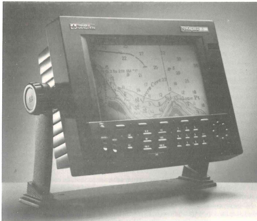
Fig. 41. NavGraphic II—an ECDIS using published nautical charts (courtesy Trimble Navigation Ltd)
