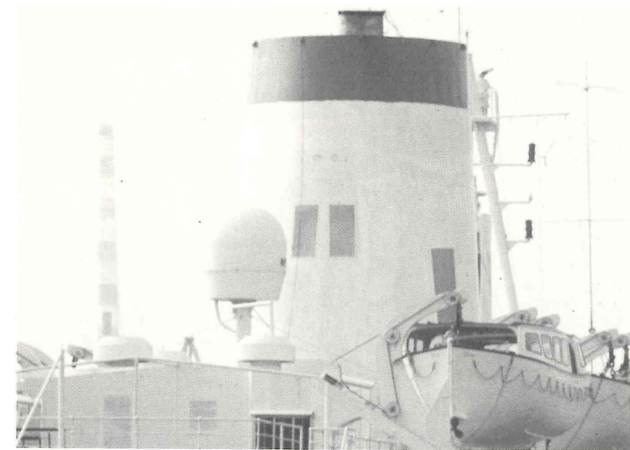
Fig. 91. A Standard A radome installation (Betsy Ross Ade) (courtesy INMARSAT)
