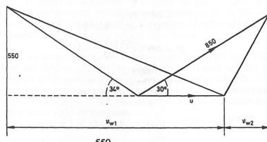
$$v_{w1} + v_{w2} = \frac{550}{\tan 34^{\circ}} + 850 \cos 30^{\circ}$$
