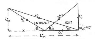
$$v_{a1} = v_1 \sin \alpha_1 = 500 \times \sin 18^\circ = 154.5 \text{ m/s}$$
