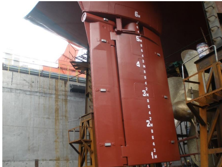
After fitting anodes and after painting
