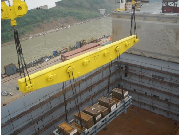
Load testing for twin crane operation
