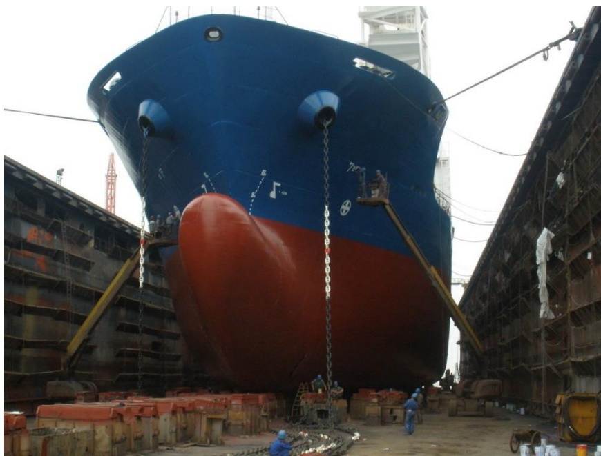
Cable ranged (look at the bottom of the dock)
