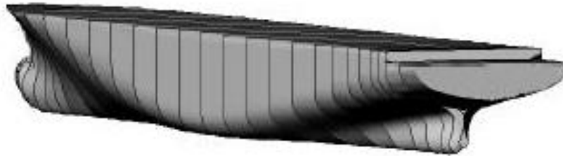
Hull form of a container ship 40
