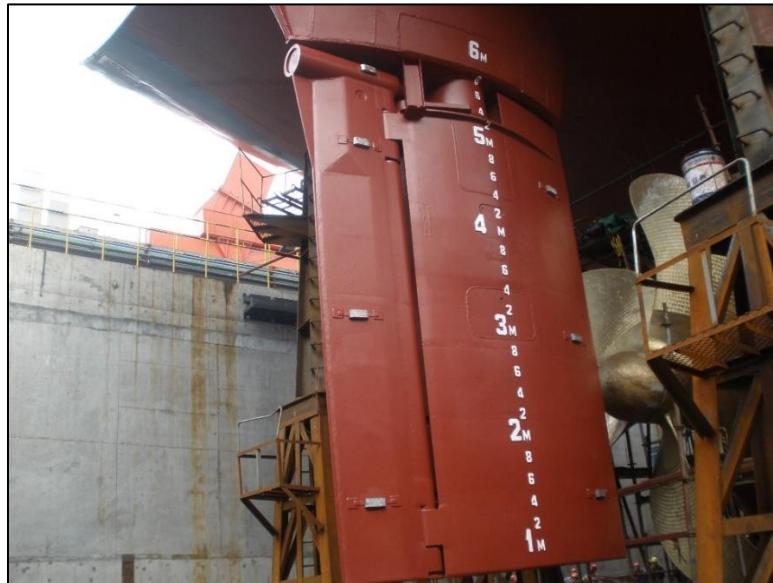
After fitting anodes and after painting
