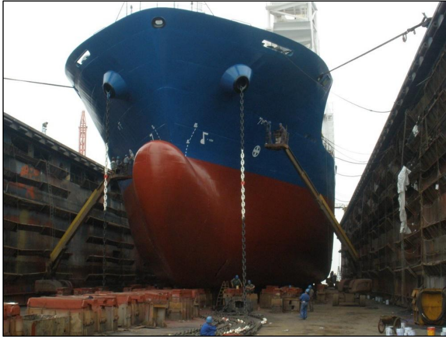
Cable ranged on the dock bottom
