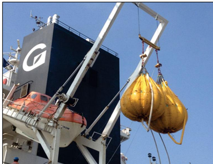
Load testing of a free-fall lifeboat falls 143
