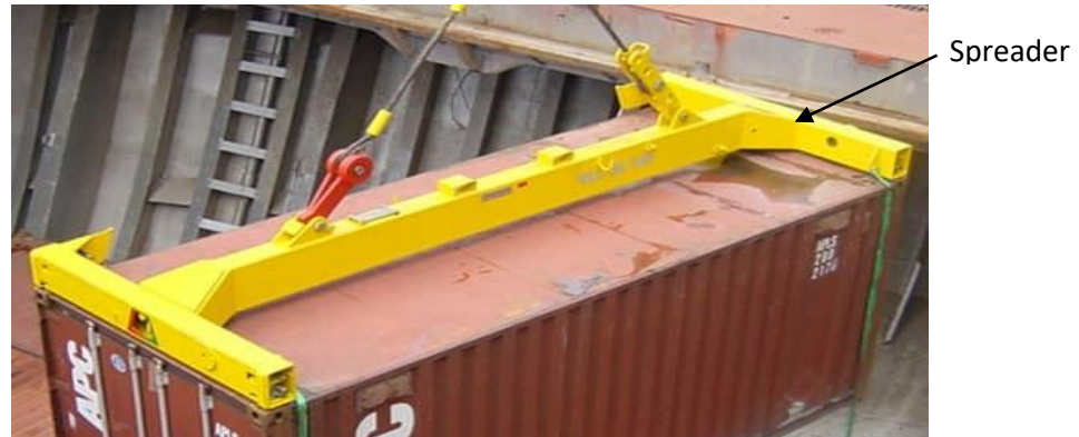
Spreader used by ships 62
