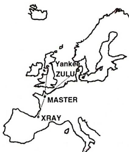
▲ Figure 2.34 Loran master with 3 slave stations
