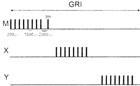
▲ Figure 2.35 Loran signals from master with 2 slaves
