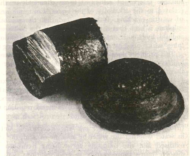
Figure 15.3 Showing how defects in a rivet head may cause it to snap
