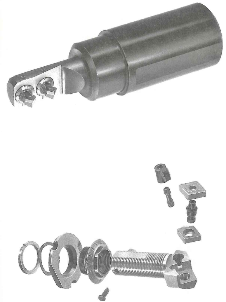
Figure 3.9b Tenthset precision boring cartridge with front adjustment of 0.0001 in.
