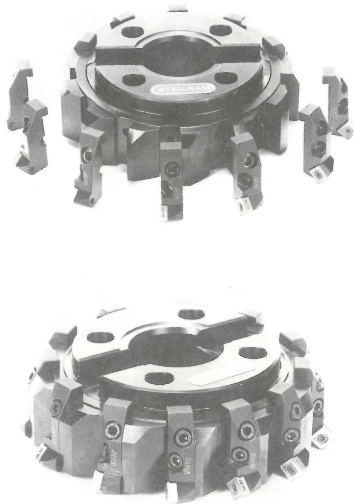
Figure 3.9c Applications of cartridges to a face milling cutter.
