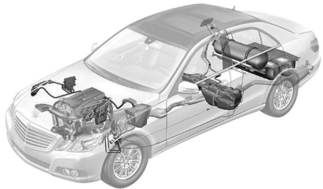
Fig. 2 Mercedes Benz E200 NGT Blue EFFICIENCY, which features bi-fuel natural gas drive [6]
