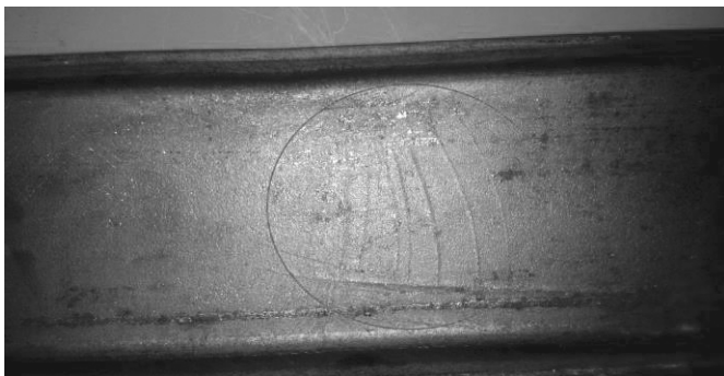
Fig. 9 Crack Initiation sites.
