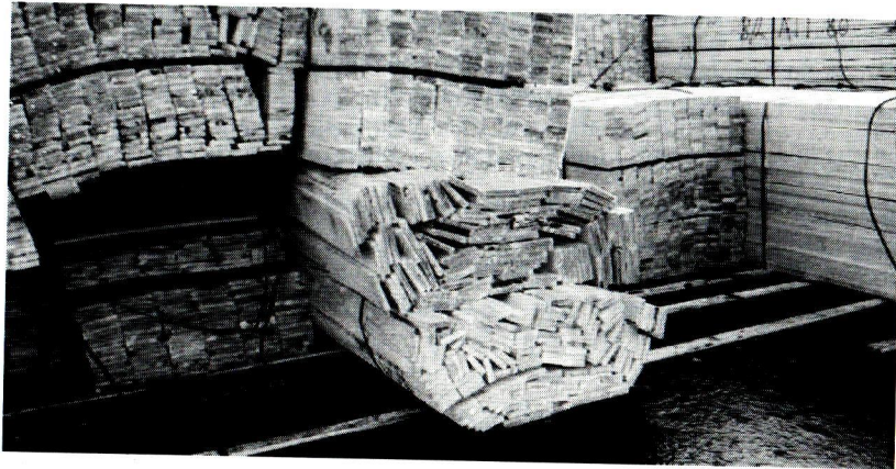
Figure 6.2 - Example of poor rigidity
